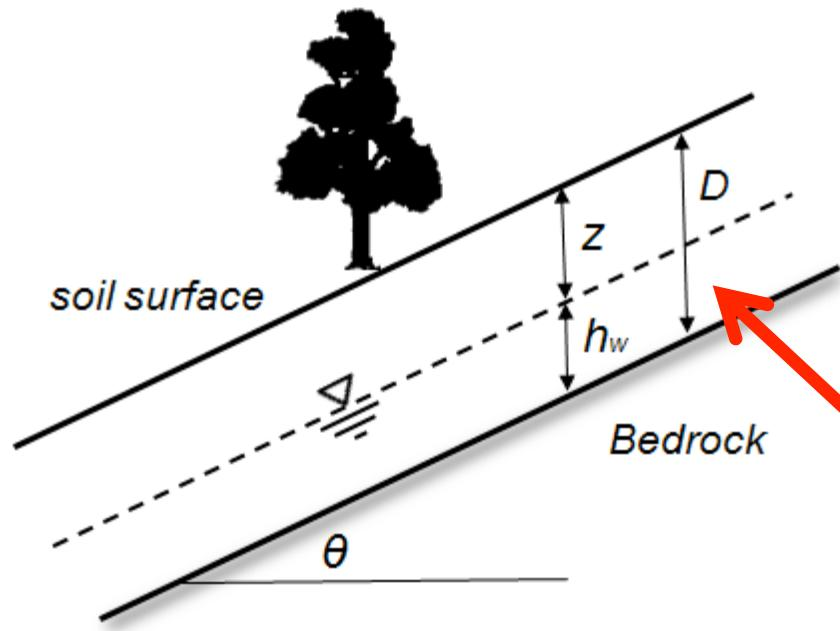
$$F.S. = \frac{c + [(\gamma_b - \gamma_w)D + \gamma_w z(t)] \cos^2 \theta \tan \varphi}{D \gamma_b \sin \theta \cos \theta}$$
